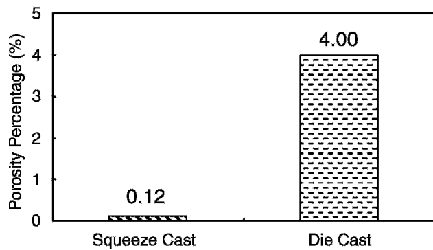
Fig. 3 Porosity levels of squeeze cast and die cast AM50 with a section thickness of 10 mm
